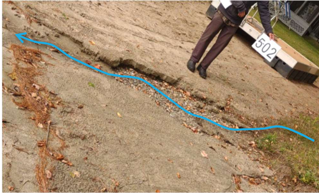
Medium impact erosion site 5-02 where runoff has caused gully erosion on a residential beach access.
