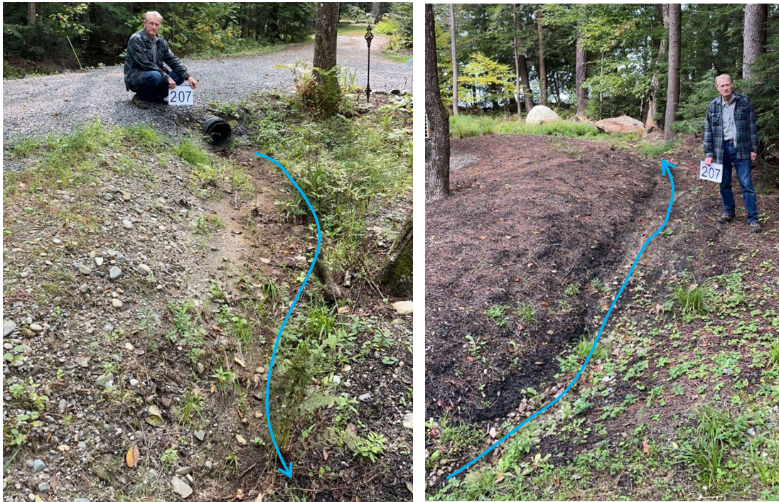
High impact erosion site 2-09 at a residential property with surface erosion (rill) and bare soil on a driveway leading down to water access.
